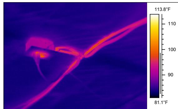
Figure 19. Thermal image of overheating wire (Figure 18).
