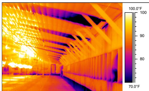
Figure 17. Cold air entering through air inlet.
