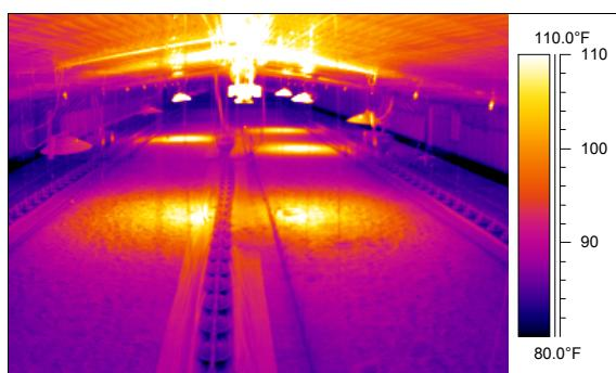
Figure 14. Floor heating patterns of two different types of radiant brooders.
