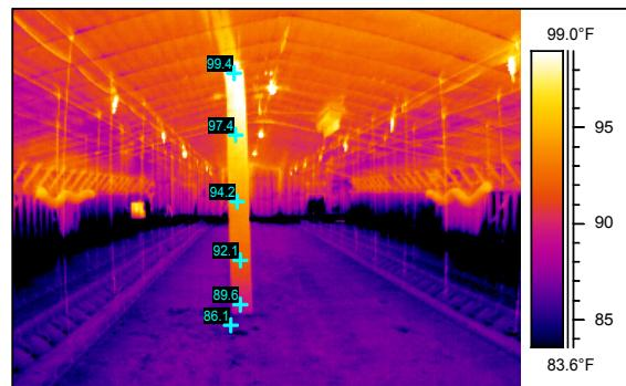
Figure 16. Temperature stratification.
