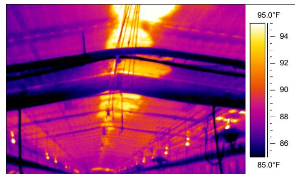
Figure 8. Missing ceiling insulation.
