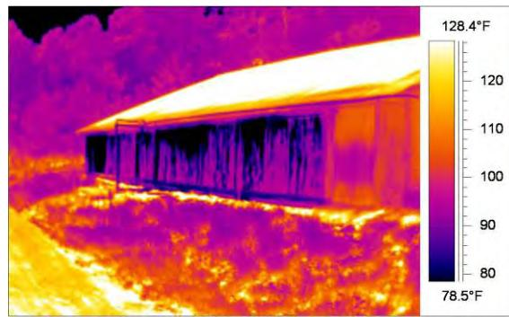
Figure 22. Thermal image of pad partially wet.
